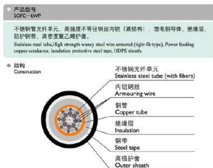
Typical Construction of Submarine Optical Fiber Composite Power Cable
